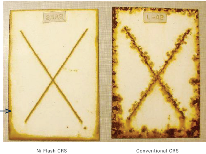
Figure 3: Four years outdoor exposure - Zinc Phosphate, two coat appliance grade paint
