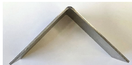
CR MartInsite® MP1300 Bend test
