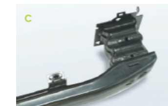
A 300 LA hot dip GI rear subframe B HR 540FB suspension arm C Bumper bracket in Dual Phase 780, Impact Absorber HSLA 300 LA
