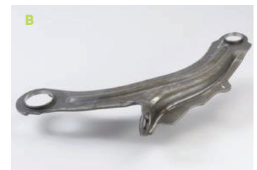
A 300 LA hot dip GI rear subframe B HR 540FB suspension arm C Bumper bracket in Dual Phase 780, Impact Absorber HSLA 300 LA
